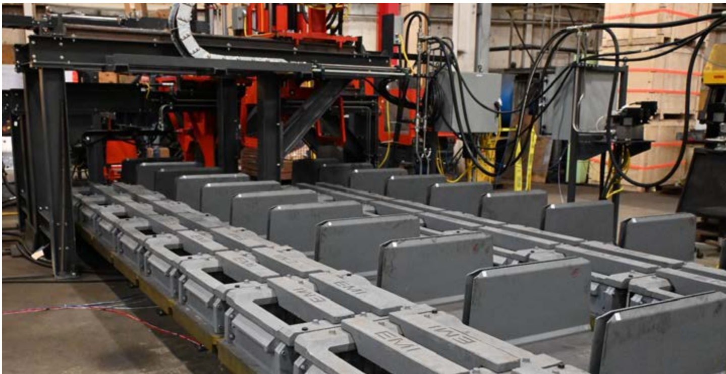
Mold handling system
