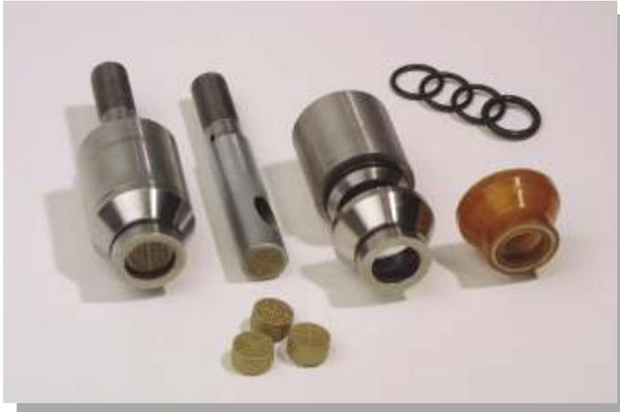
**The 3-in-1 core machine is centered on a single, straight, inner tube, a solid outer tube, and commercially available O-rings to seal the interface. All the components have been proven to be durable enough to withstand the abrasive effects of sand blowing.**
