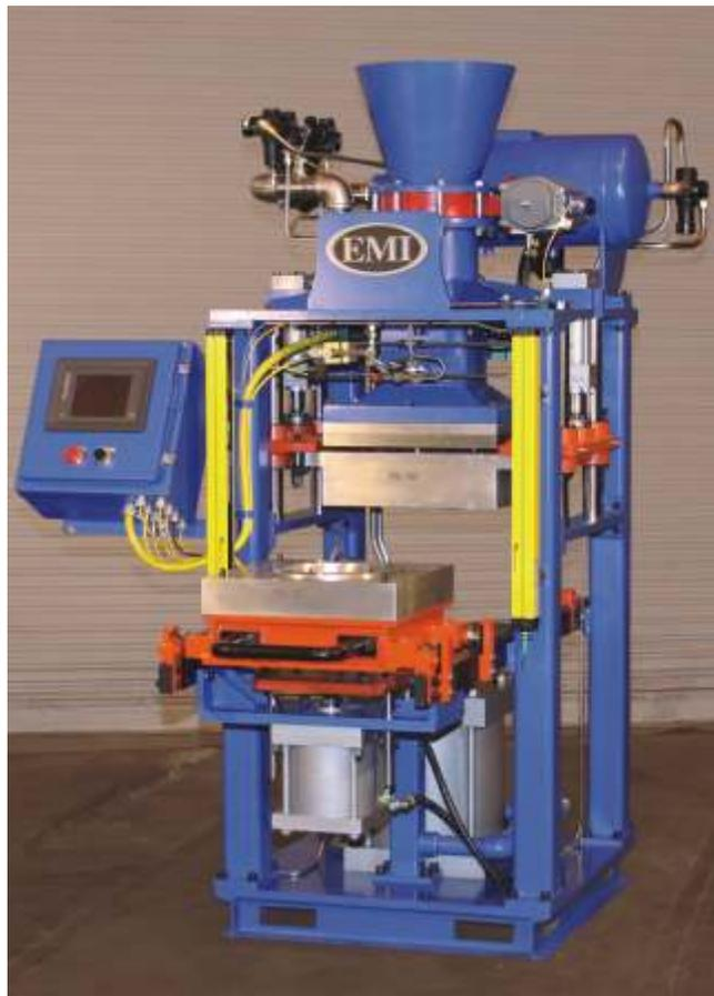
**EMI's new core machine is a pneumatic design with an air-over-oil circuit, a 75-lb blow capacity using an 18x18-inch blow plate, new tooling, and a drag roll-out cart with an external ejection system.**
