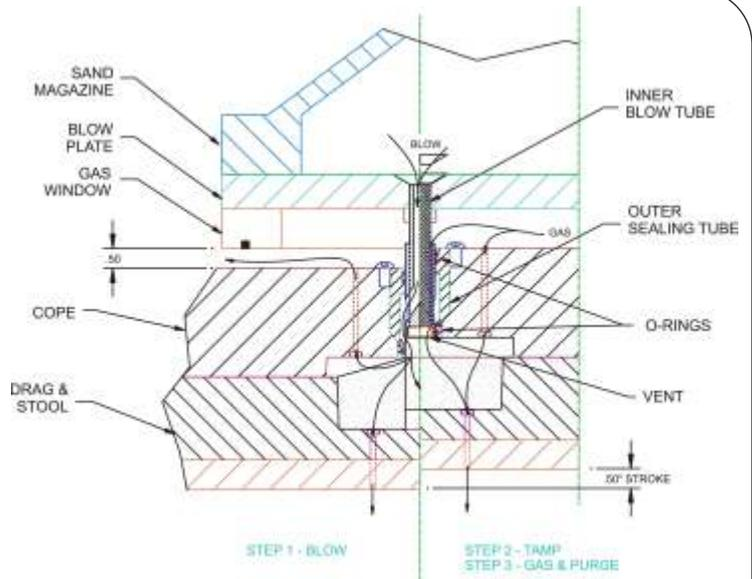
**EMI theorized that leaving a slight back-pressure in the blow head during gas and purge, would prevent undesired migration of catalyst into the inner tube. A back-pressure regulator valve was installed in the blow circuit.**
